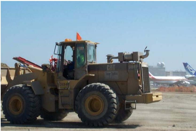
Figure 1.2-6: Caterpillar Loader E03412 Outfitted with ECS Purifier VDECS
