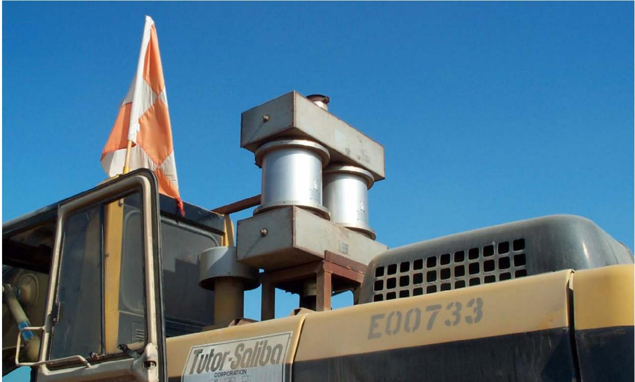
Figure 6-4: E00733 Was Found to have VDECS Sensors Not Hooked Up
