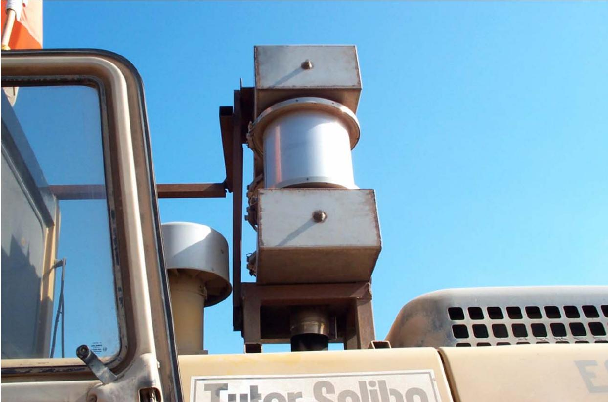
*Figure 6 -3: Caterpillar Excavator E00733 Equipped with ECS Purifilter VDECS*
