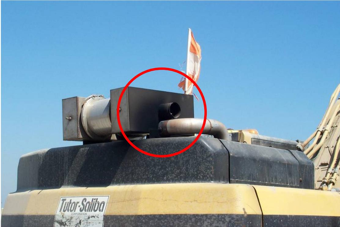
*Figure 6.2-8: E00732 Was Found to have VDECS Not Hooked Up*
