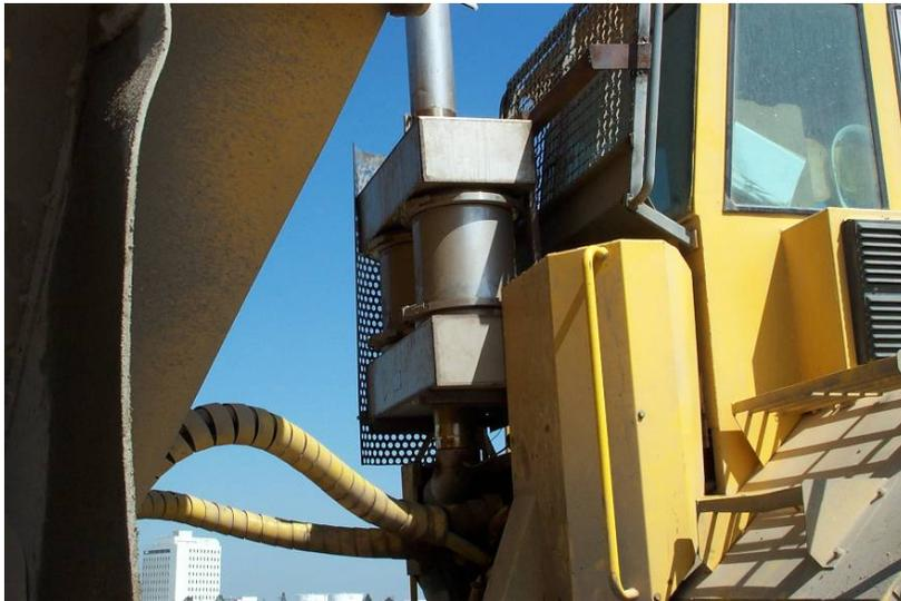
*Figure 1.2-4: Volvo Articulated Dump Truck E00234 Outfitted with ECS Purifilter*
