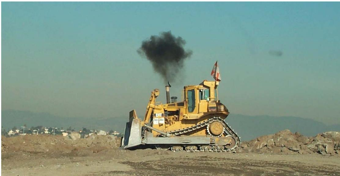
*Figure 6.2-6: CAT Dozer E00349 – Vehicle Reported as Emitting Excessive Soot*
