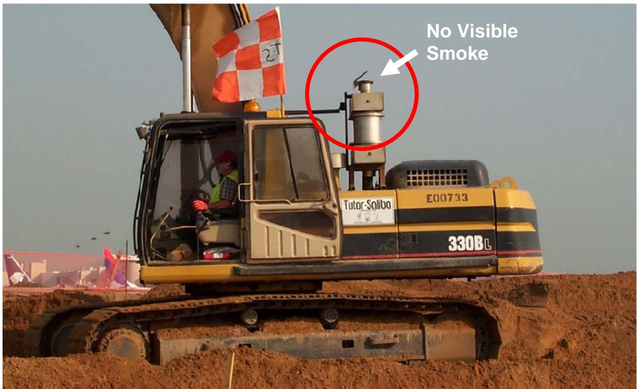
Figure 6-5: Caterpillar Excavator with Functioning VDECS
