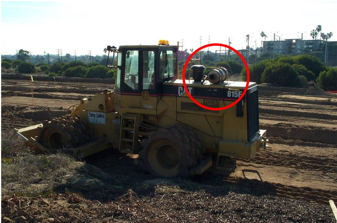
Figure 6.2-10: CAT Compactor E00651 is Equipped with an ESC Purifilter VDECS
