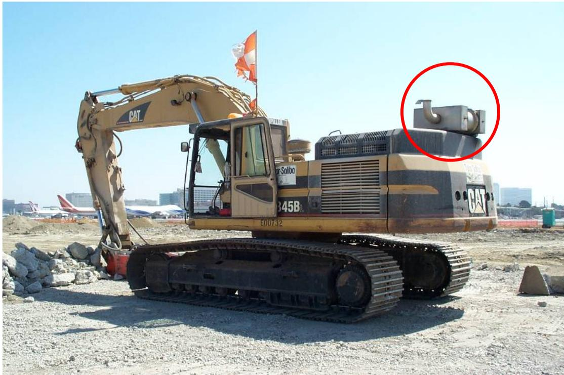
*Figure 6.2-7: Caterpillar Excavator E00732 Equipped with ECS Purifilter VDECS*
