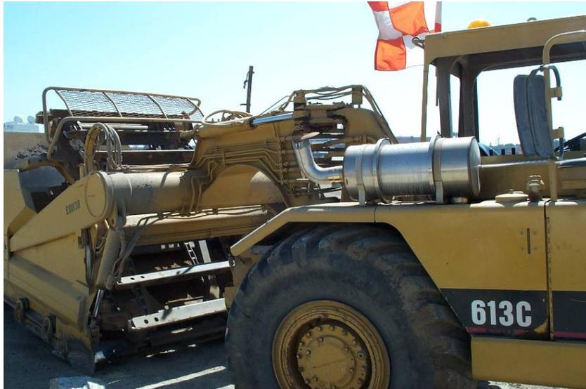
Figure 1.2-5: Caterpillar Scraper E00138 Outfitted with ECS Purifier
