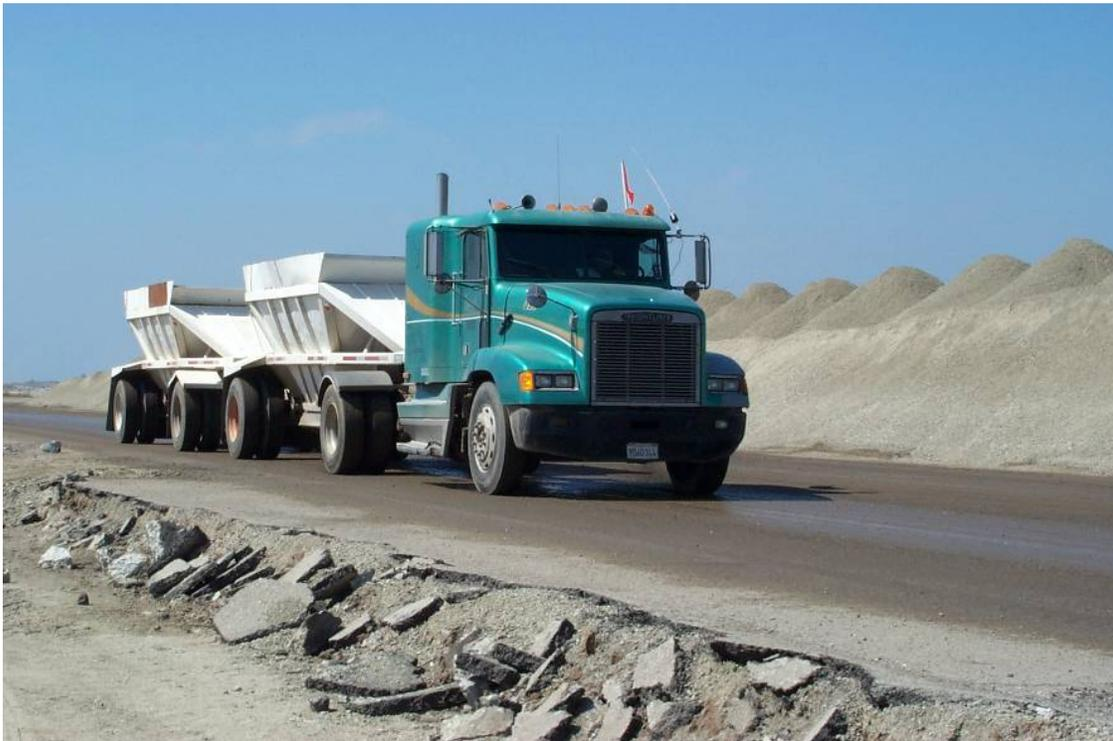
*Figure 6.2-12: Haul Roads are Kept Wet to Reduce Fugitive Dust Emissions*
