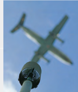
Microphones, like the one shown here, measure the level of noise created by aircraft operating at LAX.
